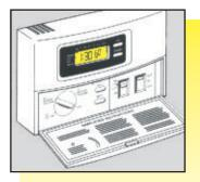
Install clock thermostat with a 5 degree setback at night.
